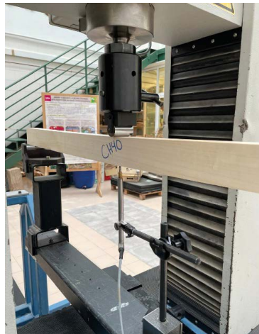
Figure 4. Non-destructive static center-point bending test.
