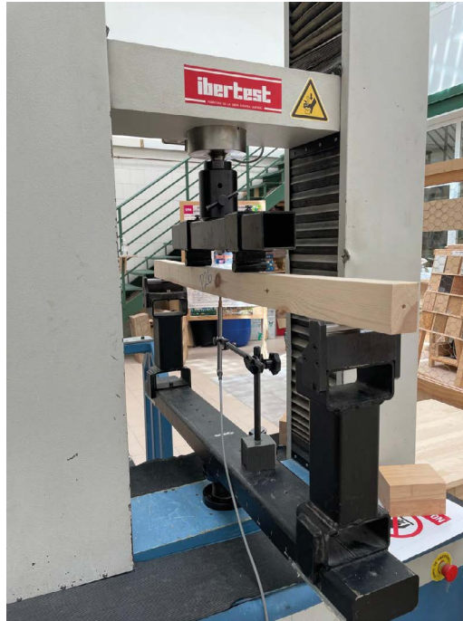
Figure 6. Four-point static bending test according to EN 408:2011.
