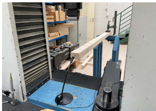
Figure 3. Transverse vibration testing of a cantilever beam.
