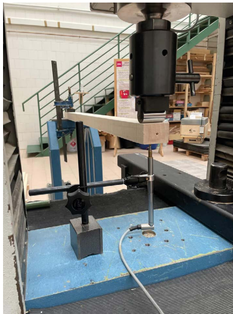
Figure 5. Non-destructive static bending of a cantilever beam.
