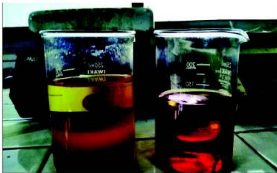
Figure 10. Fatty acid methyl ester (FAME): (a). esterification (b) biodiesel.
