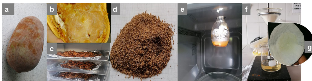
Fig. 1 Step-by-step photographic overview of the microwave-assisted extraction procedure for obtaining pectin from cupuassu pod husks: (a) cupuassu fruit, (b) Pod husk, (c) drying stage, (d) milling and sieving, (e) MAE-treated samples, (f) filtration of the extract, (g) pectin product
