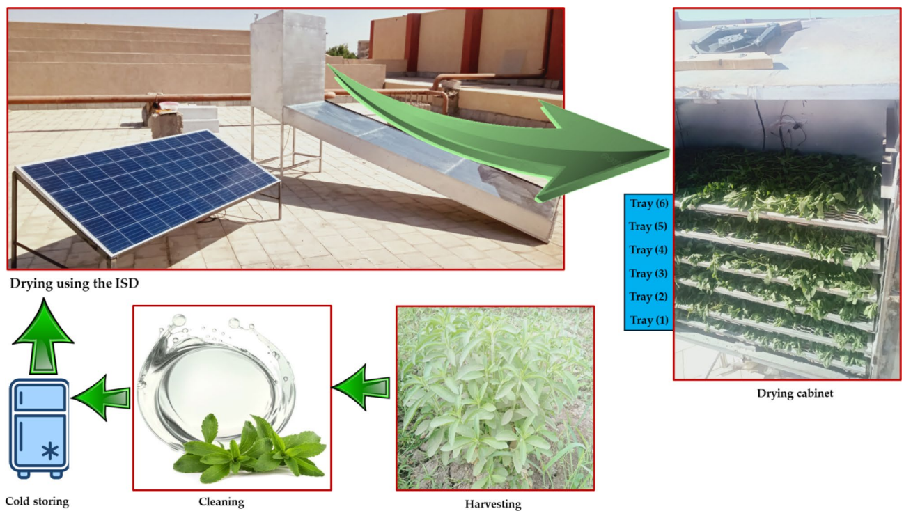
Fig. 2. Diagrammatic representation of the stevia sample preparation and drying workflow in the PVT-ISD system.
