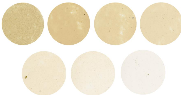
Figure 5. Laboratory sheets performed with different pulp proportions. Correspondence, from left to right: 100% of Phytolacca fibers, 90% of Phytolacca fibers and 10% of commercial pulp; 70% - 30% ; 50% - 50%; 30% - 70%; 10% -90% and 100% of commercial pulp.
