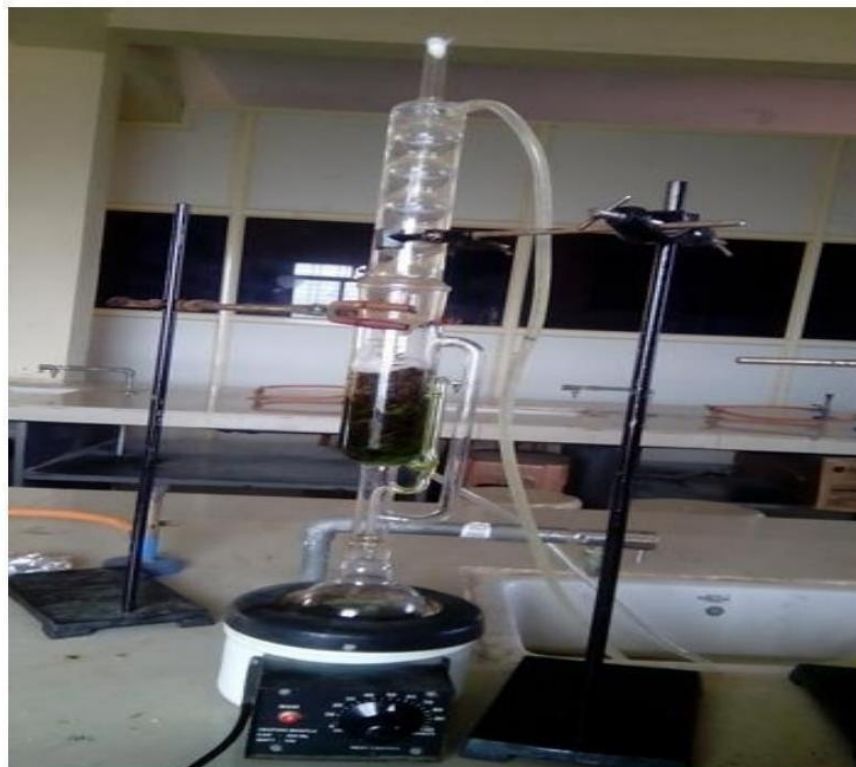
Fig. 3: Extraction Procedure by Soxhlet
