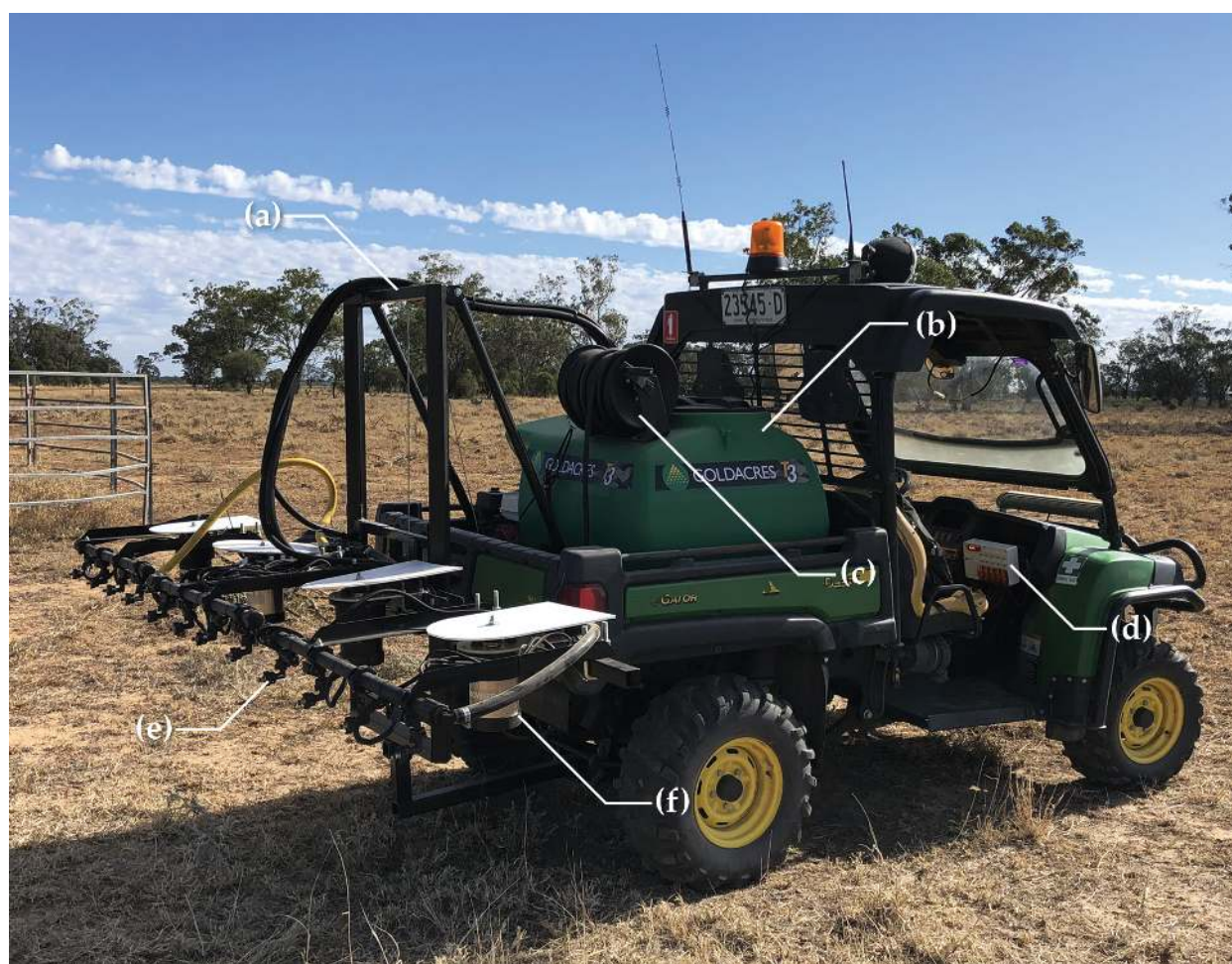
Figure 4. A John Deere Gator UTV with an installed three metre AutoWeed spot spraying system, including: (a) a winch and frame for electronic height adjustment, (b) a 300 L Goldacres T3 tank and a 20 L/min diaphragm pump with a Honda GX120 engine and manual pressure regulator, (c) a spray handgun and reel for manual spraying, (d) an AutoWeed control box to monitor unit operation, (e) a 1" wet boom with twelve TeeJet solenoids, nozzle bodies and Turbo FloodJet spray nozzles, and (f) four AutoWeed detection units.
