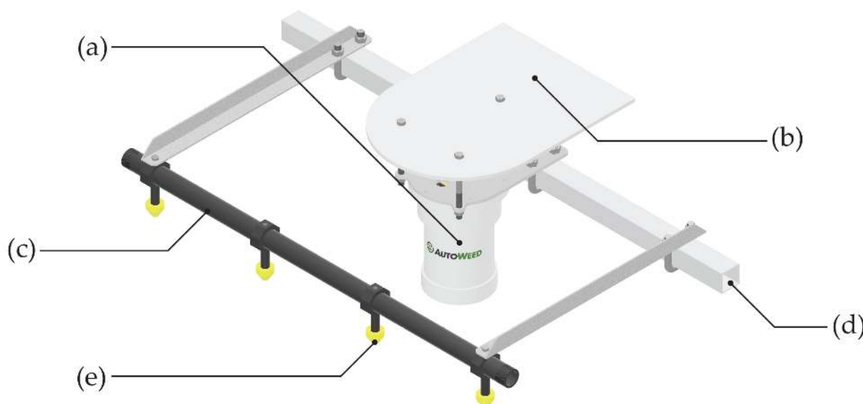
Figure 3. AutoWeed’s proprietary weed detection and spraying boom mount design for a 1 metre boom section, including: (a) the AutoWeed detection unit, (b) a protective sun shade, (c) a 1” wet boom, (d) a 40 × 40 mm steel hollow section frame, and (e) TeeJet solenoids and nozzle body adaptors.
