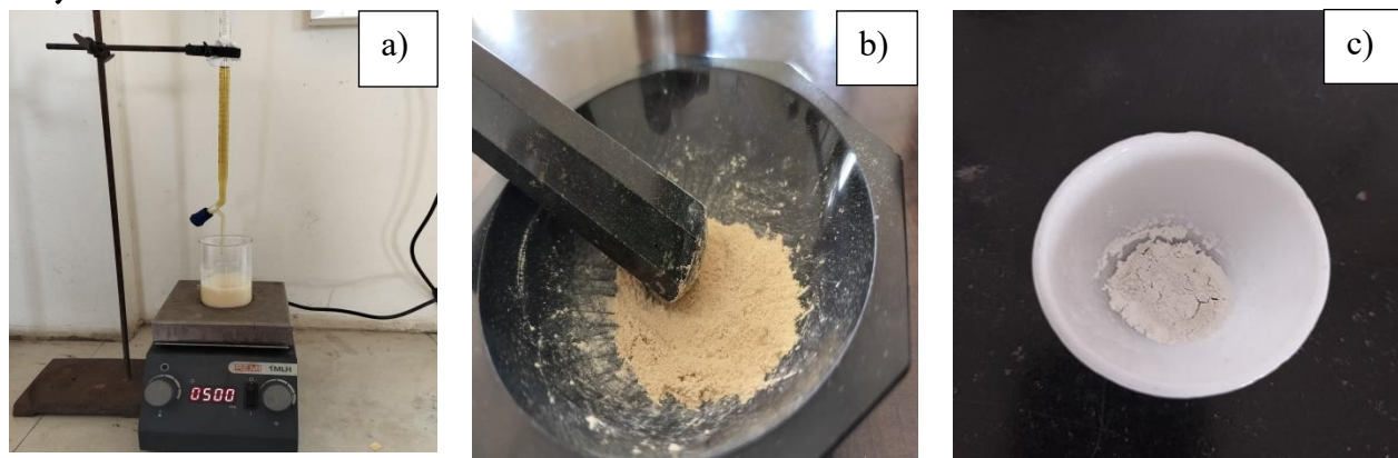
Fig 2. a) Addition of Plant extract to Precursor b) TiO 2 NPs c) After Calcination TiO 2 NPs
