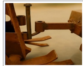
Fig 5: Motor-to-chassis mounting arrangement.
