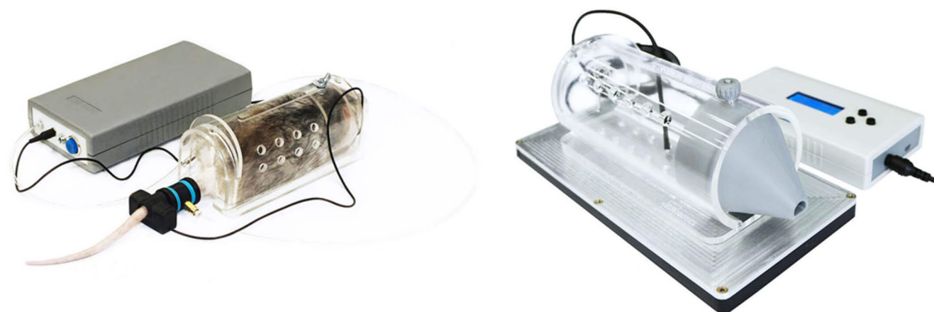
Fig. 2 Experimental device “Sistola” (Neurobotics, RF) for noninvasive recording of arterial blood pressure in the blood vessel of the tail artery in rats
