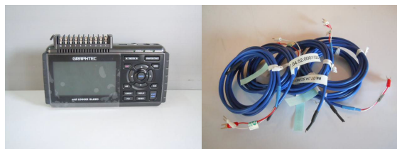
Fig. 4 Graphtec data loggers and thermocouple wires
