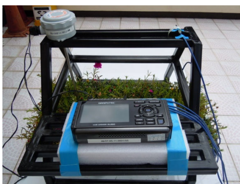
Fig. 8 The temperature measuring of purslane tray
