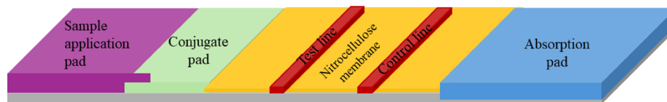
FIGURE 5 The basic structure of the LFIA test strip (modified image based on Xu et al., 2022).
