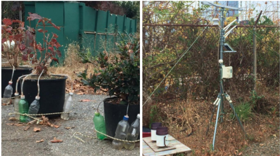
Figure 6- Stemflow Collection System and HOBO Weather Station
