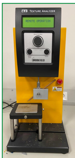
Figure 4 – Point (graphite) breaking test machine setup
