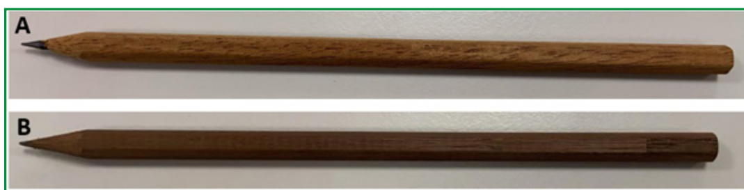
Figure 5 – Successfully produced pencils from thermally modified iroko (A) and ash (B)
