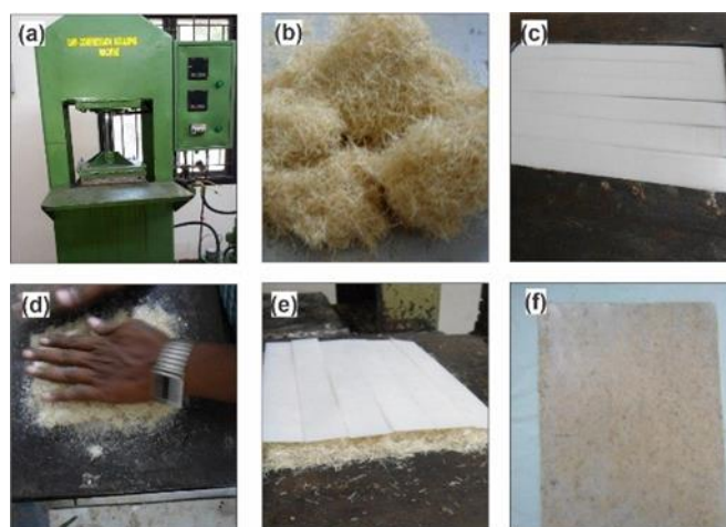
Fig. 2 Making of PCL/SRF biocomposite Panel (a) Compression moulding machine b Chopped SRF c PCL strips d SRFs on PCL strips e Arrangement of PCL strips and SRFs and f Biocomposite panel
