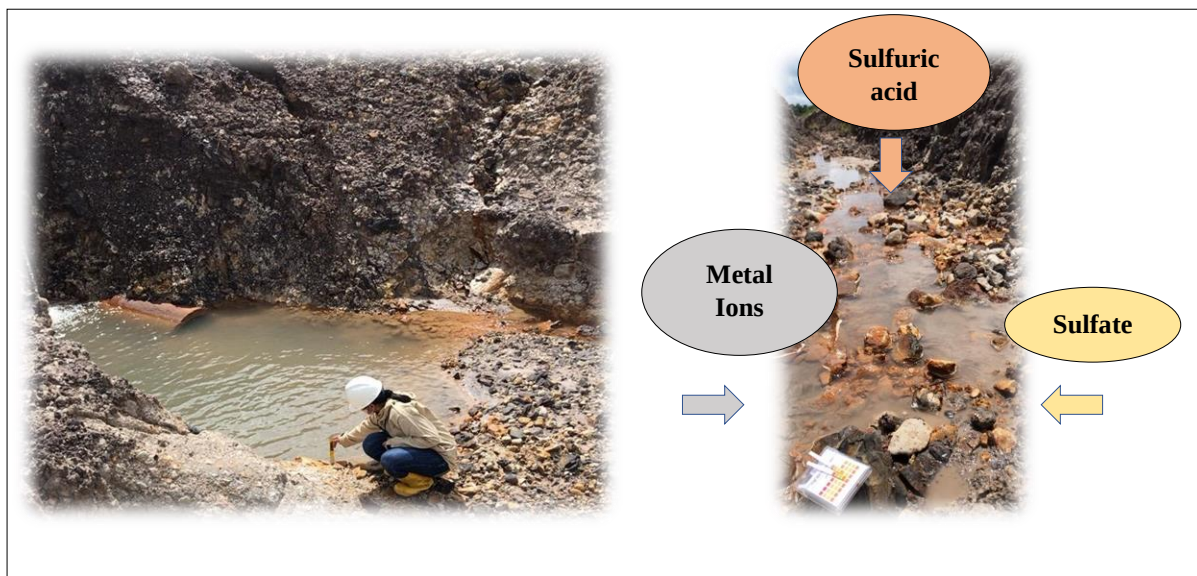
Figure 2. AMD from High-Fe and Mn in Coal Mining Area (documentation, 2024)
