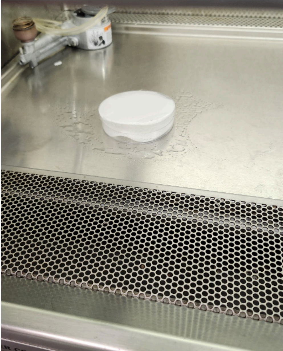
Photograph of prepared petri dish in a laminar flow hood with its lid cracked to allow ethanol and water to evaporate out of the filter paper.
