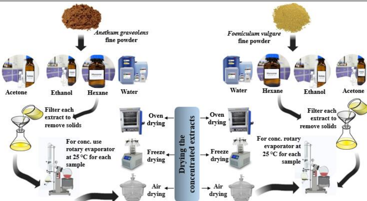
Figure 2: Schematic illustration of solvent-based extraction of A. graveolens and F. vulgare seed powders using acetone, ethanol, hexane, and distilled water
