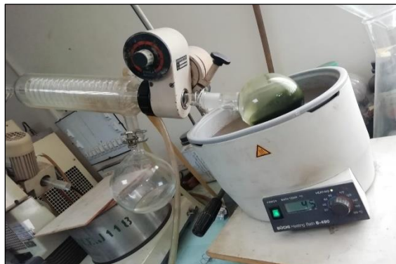
Figure 4: Rotary evaporator used in removing solvents and concentrating extracts.
