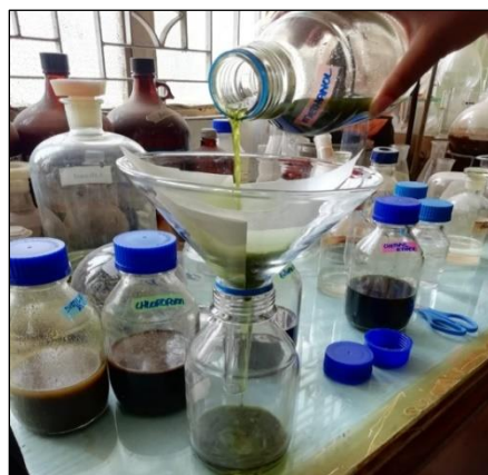
Figure 5: Filtration process involved in extraction where the marc is separated from the liquid extract.
