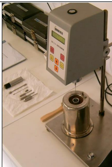
[ FIGURE 11: MEASURED USING A BROOKFIELD VISCOMETER AT ROOM TEMPERATURE ( 25 \pm 1^\circ\text{C} ) ]
