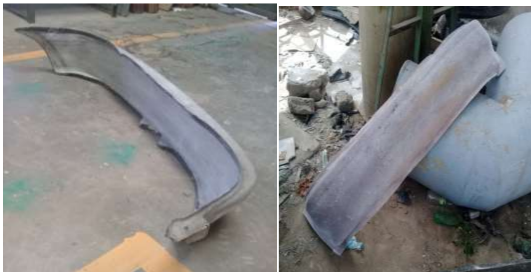
Plate VII: Fabricated bumper mould, (Inner and outer surface)
