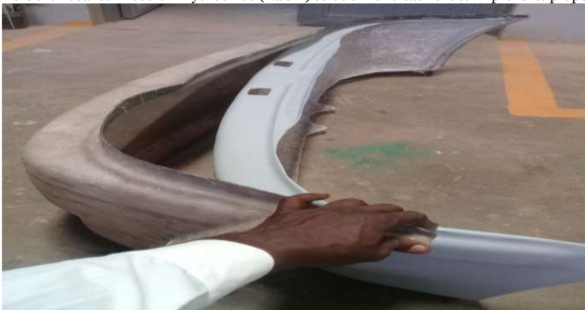
Plate IV: Removal of cast bumper from the mould.
