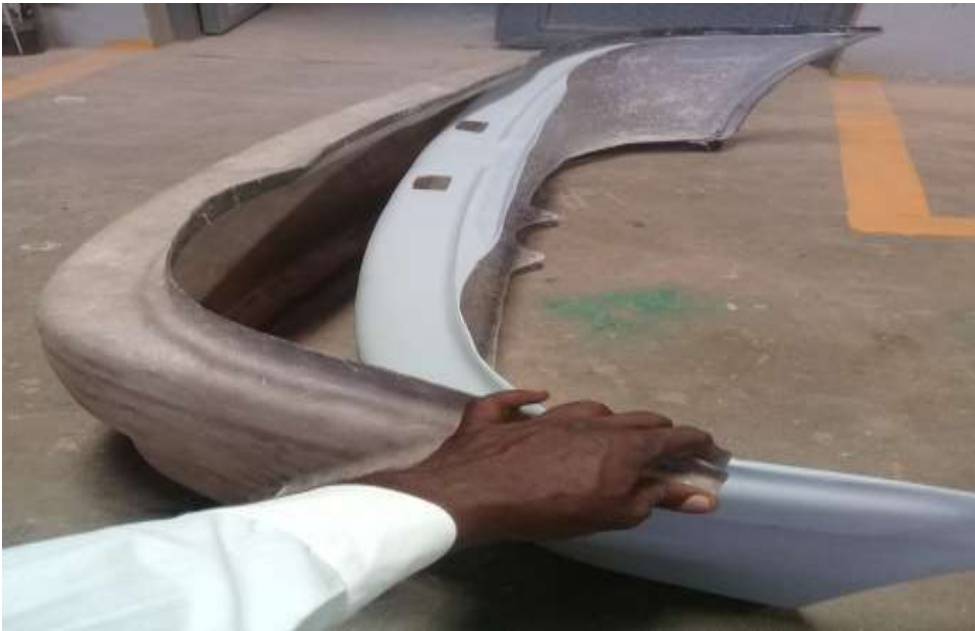
Plate X: Removal of cast bumper from the mould.
