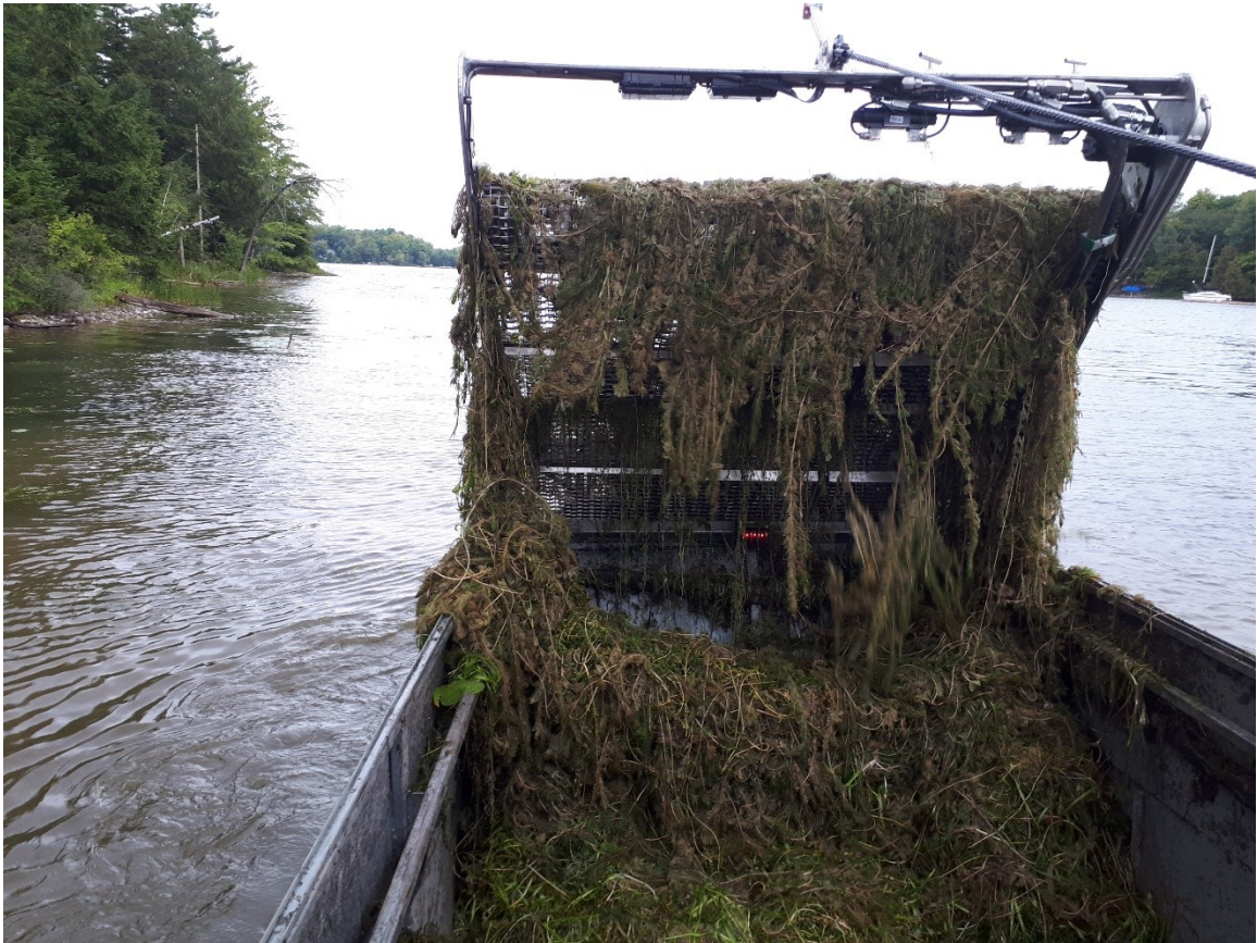
Figure 2-3. Rideau Aquatic’s custom harvester barge is an example of a mechanical cutting system used in macrophyte control. Here the conveyor and sickle are deployed and are cutting a swathe through an M. spicatum patch on Otter Lake in September 2019.
