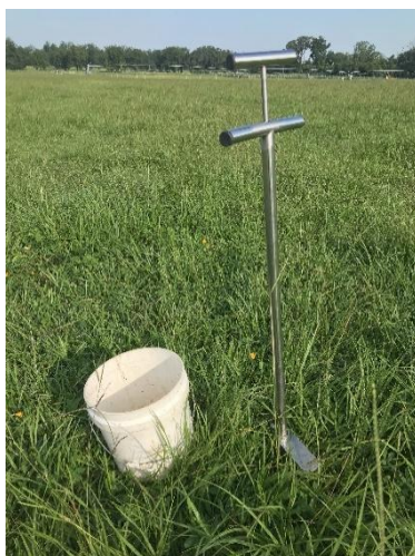
Figure 5.1 Apparatus for soil sampling at the site of the assay (Personal file).
