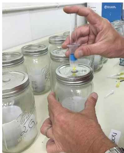
Figure 5.3 Gas collection to determine the ^{13}\text{C} from \text{CO}_2 during assay (Personal file).
