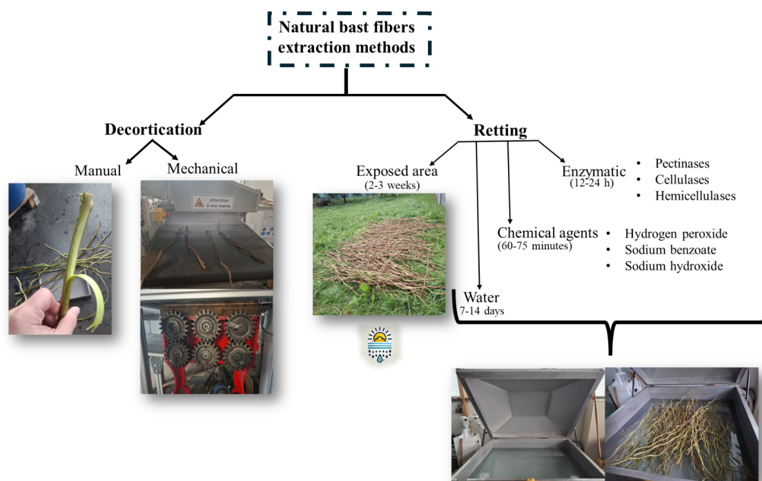
Fig. 5 Schematic representation of the different methods for bast fibers extraction [33] . Images obtained at Lorraine University (LERMAB Laboratory). The hop biomass used in this study was sourced from the agricultural center in Obernai, Alsace.
