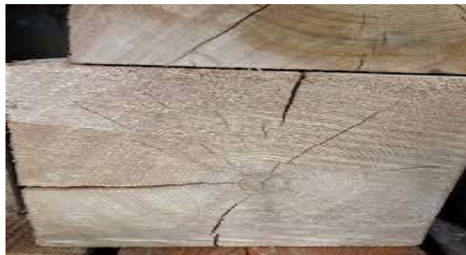
Plate 6: Wood with checks and splits when exposed outdoor
