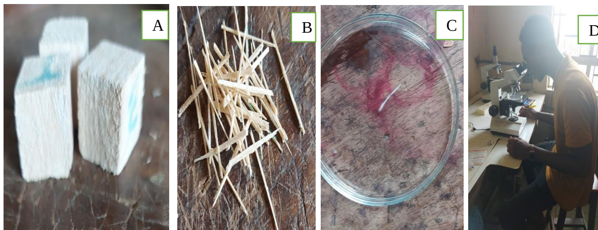
Plate 11: A: sample size for anatomical test B: chipped fibres C: Maceration of fibres D: Measurement of fibres under the microscope
