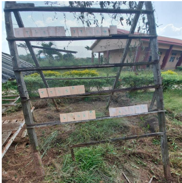
Plate 13: Samples set out on the weathering panel
