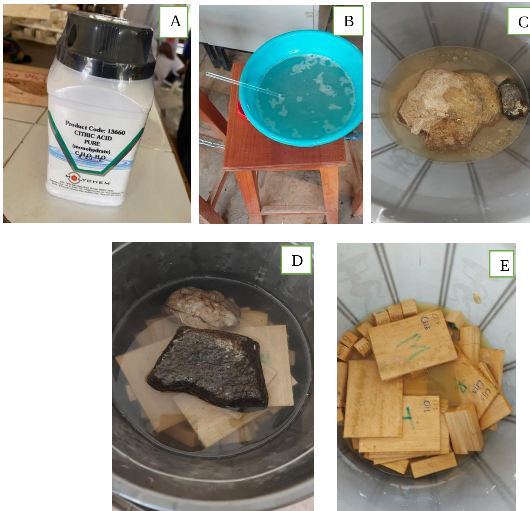
Plate 10: A: Citric acid pure B: preparation of the chemicals into solution C: Dipping of the wood samples in prepared citric acid D: Dipping of the wood samples in prepared calcium chloride E: Dipping of the weathering samples in the prepared chemical solution
