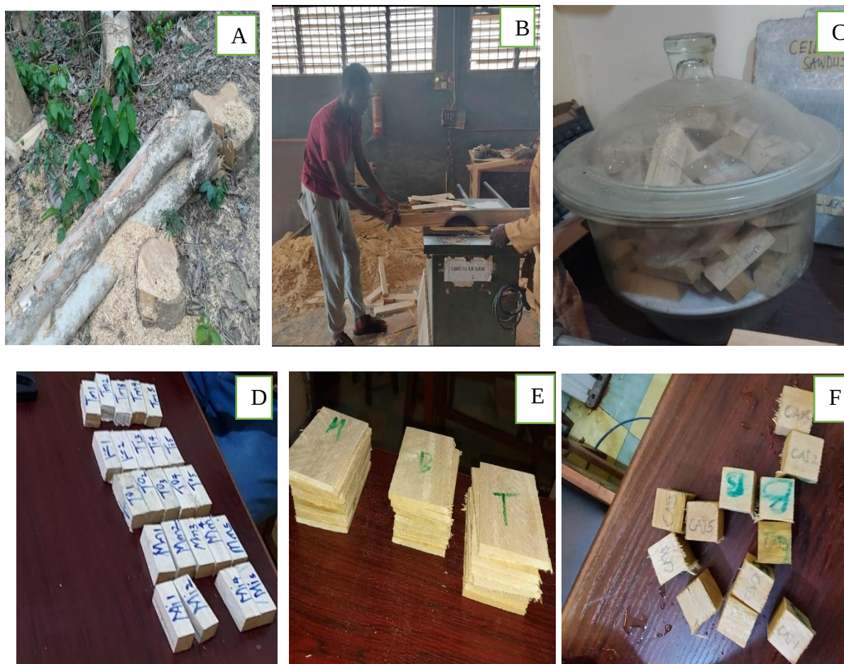
Plate 9: The collection and preparation of wood samples; A: G. arborea tree harvesting using chain saw B: Conversion of billets with circular saw C: Conditioning of wood D,E and F: Converted defect free wood samples
