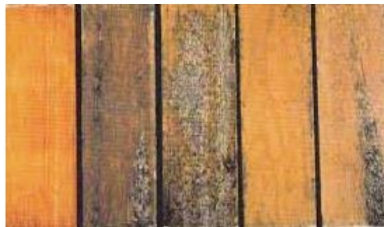
Plate 5B: Wood exposed to UV light
