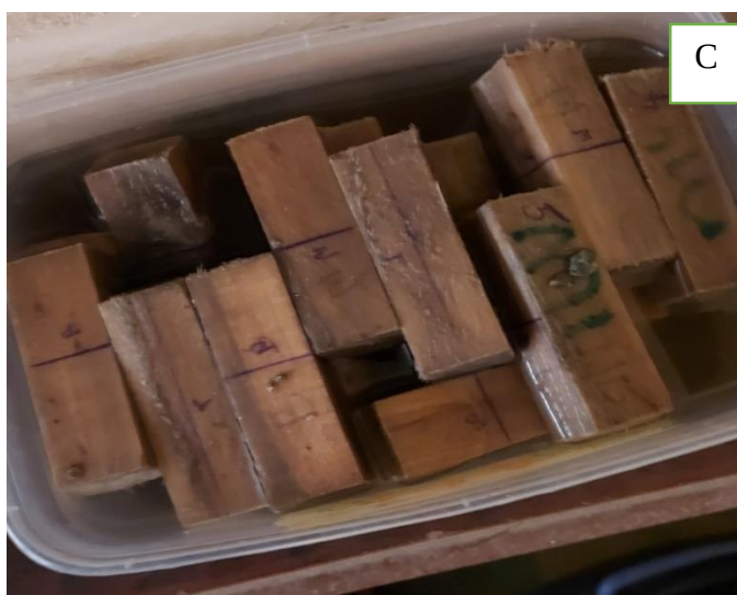
A: Weighing of wood samples B: soaking of wood samples C: wood samples after 72 hours of soaking.
