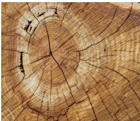
Plate 4A: Cracks in wood
