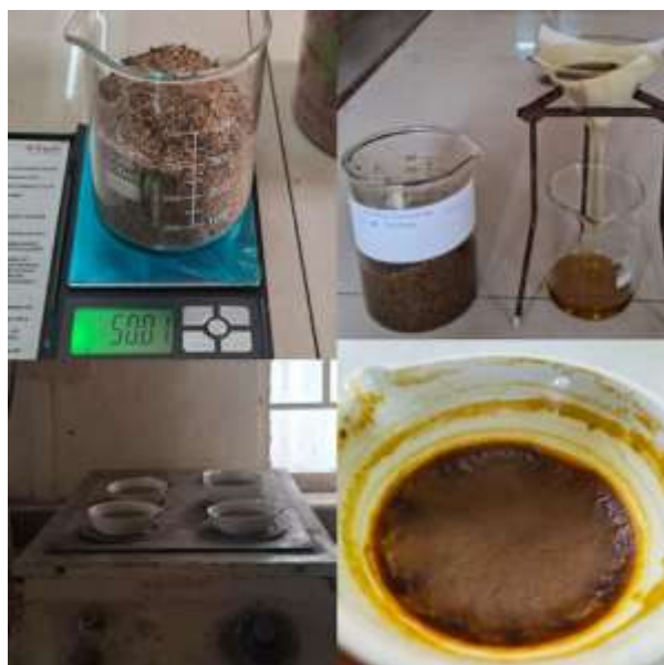
Figure 3. Extraction process of Polianthes tuberosa flower extract
