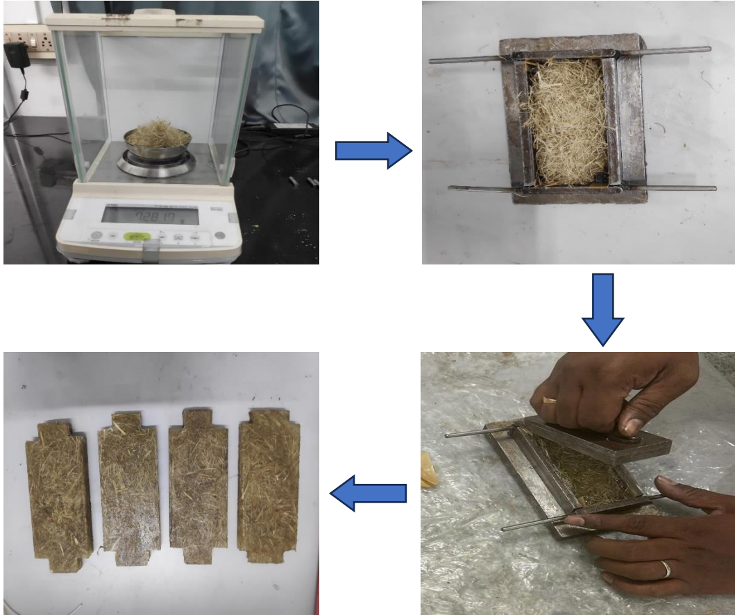
Figure 2: AIF reinforced Composites Fabrication
