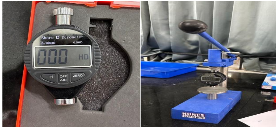
Figure 3: Experimental setup of Shore D hardness Measurement
