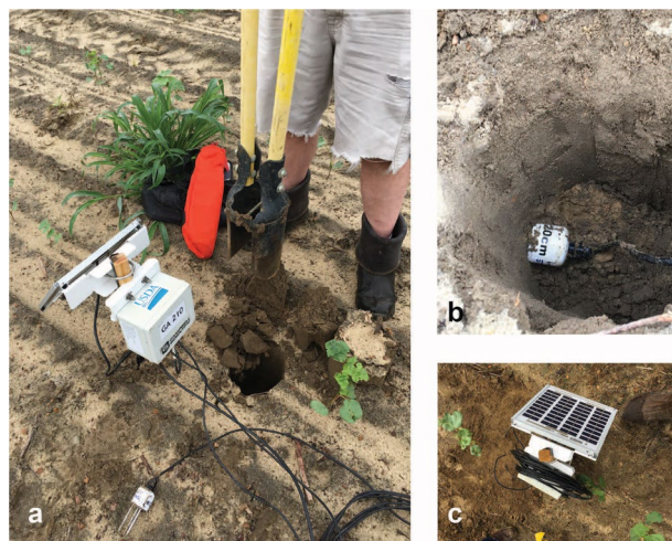
Fig. 3 Photographs showing installation of soil moisture sensor (a), placement of sensor at 20 cm depth (b), and final installed in situ sensor (c).
