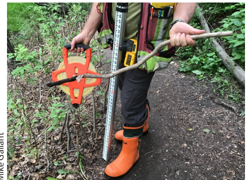
Dead live cutting planted too shallow into anoxic soils
