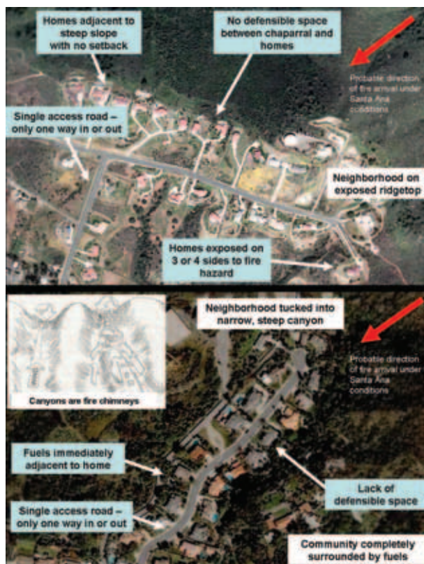
Figure 2. Many California housing tracts violate basic principles of fire safety in high-fire-hazard areas. Topography is a major factor influencing home safety. Homes built atop topographic high points require setbacks from steep slopes, as wind-driven flames and convective heat can impact these homes directly. Homes in natural chimneys are highly prone to fire-loss, as narrow canyons and saddles act as wind tunnels.
