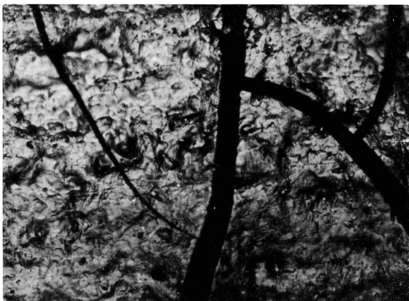
Fig. 3(b) Crack pattern developed after microwave exposure for 240 seconds x 250.
