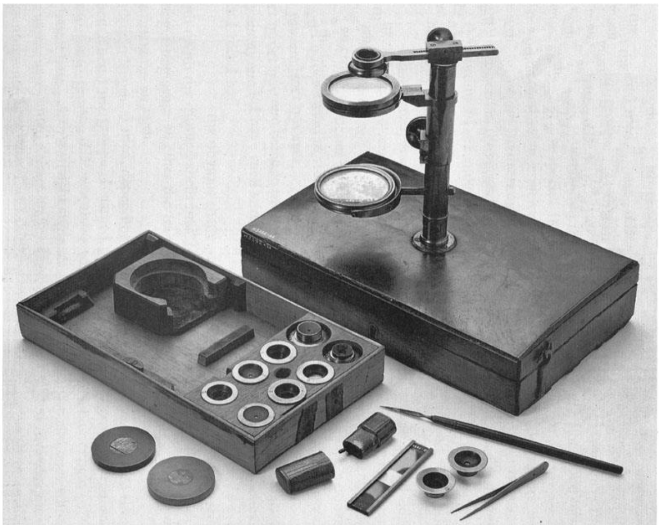
Ellis Aquatic Microscope, London, c. 1760. This simple microscope was designed by John Ellis for his pioneering research in marine biology; Banks and Solander took four of them on the Endeavour. Photograph by Jaime Plaza, Royal Botanic Gardens, Sydney.
