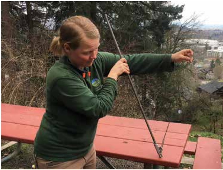
Fig. 3. Using a rod to drive the anchor into the ground.
