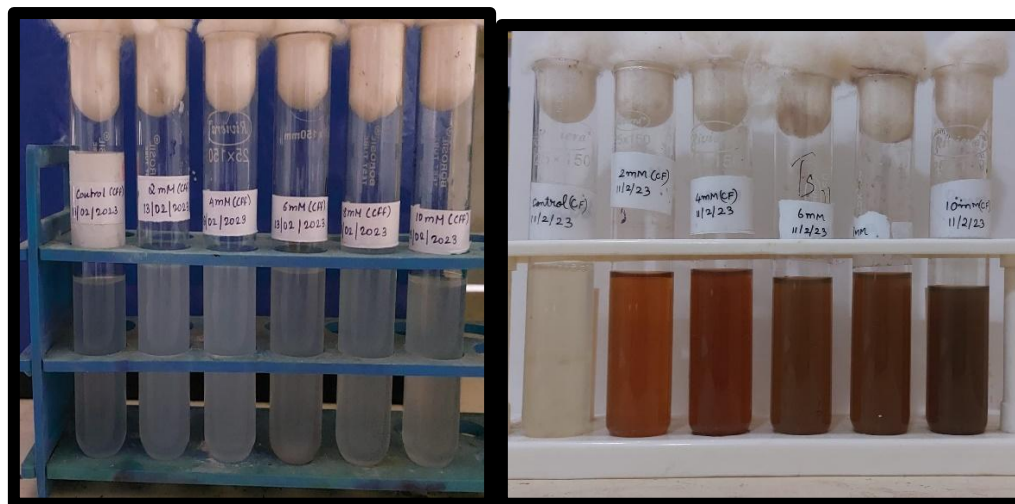
Fig. 6 A) Pichia kudriavzeii extract and \text{AgNO}_3 . B) synthesized silver nanoparticles
