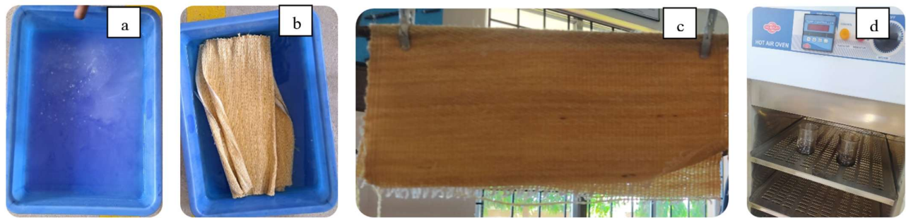
Fig.3 Activities conducted during chemical treatment and microwave irradiation (a) NaOH -aqueous solution (b) fiber soaked in aqueous solution (c) open air-drying (d) microwaved for one hour
