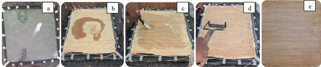
Fig.4 Activities carried out during laminate preparation (a) Glass mold (b) Incorporation of NN filler-epoxy mixture at a varying weight percentage (0, 5, 10, and 20 wt%) (c) Disseminating the mixture (d) A roller utilized during hand layup process (e) prepared laminate
