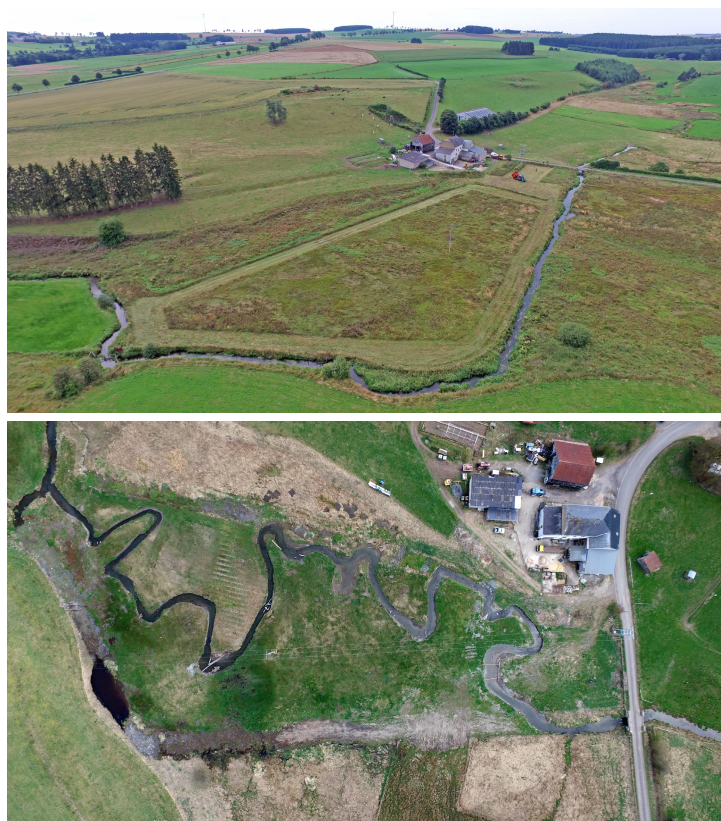
Fig. 3. The remeandering of the Trèterbaach as seen from above.
