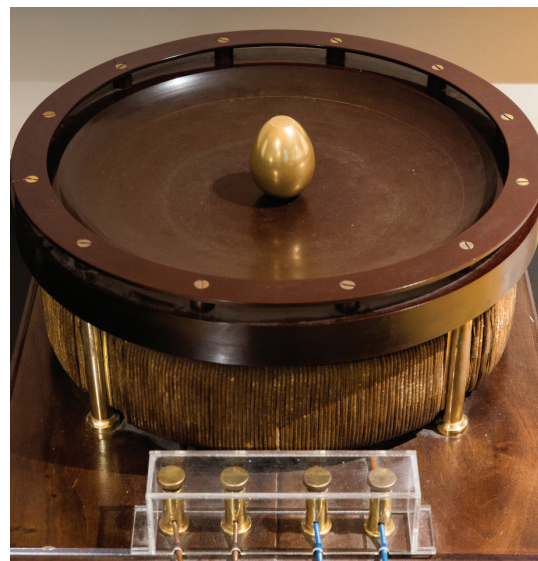
Photo 2: Induction motor with Egg shaped rotor.
