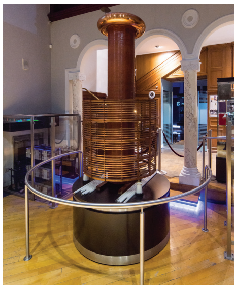
Photo 1: Tesla Oscillating Transformer 500 kV.
