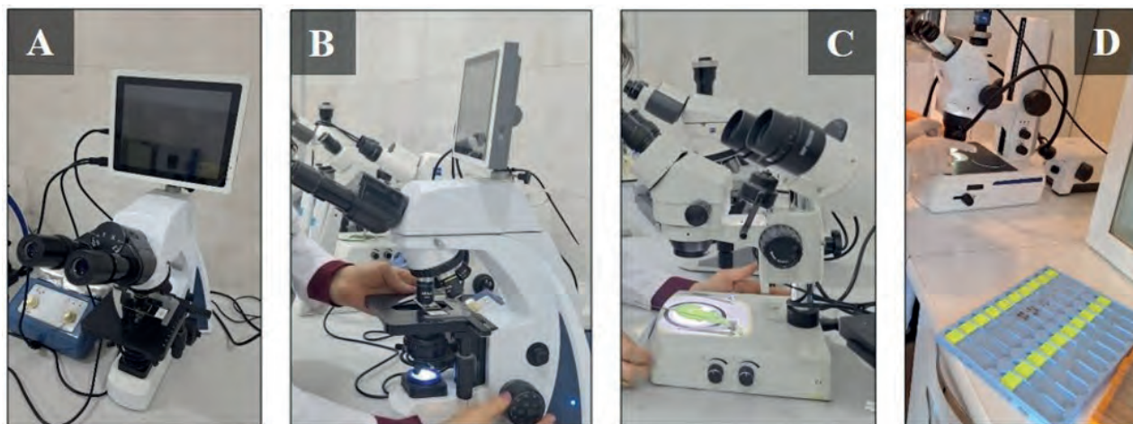
Figure 4. Optical and stereoscopic microscopes used. A, B: LCD Dijital Mikroskop NLCD-307B; C: Steroscope Zeiss Stemi508; D: Stereo YK-SM067B2.
