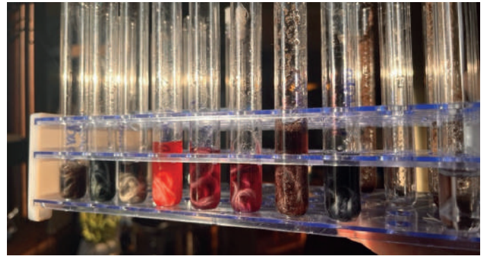
Figure 2. Small-scale test samples from aspen pollen—examining color shifts using different pH solutions in combination with alum—a potassium salt used for pickling.
