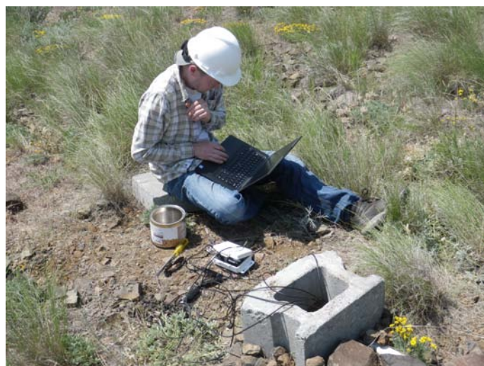
Figure 9. Dr. Eric Graham of CWU sets up the datalogger (foreground) to continuously record temperature and soil moisture. PHOTO: RON BOCKELMAN
