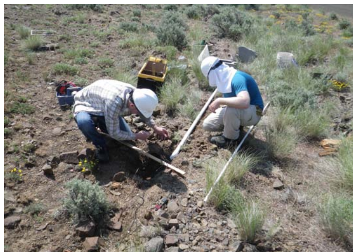
Figure 8. Team members installed soil moisture and temperature sensors below the ground surface, after first running the cables through a PVC pipe to prevent rodents from chewing them. PHOTO: RON BOCKELMAN
