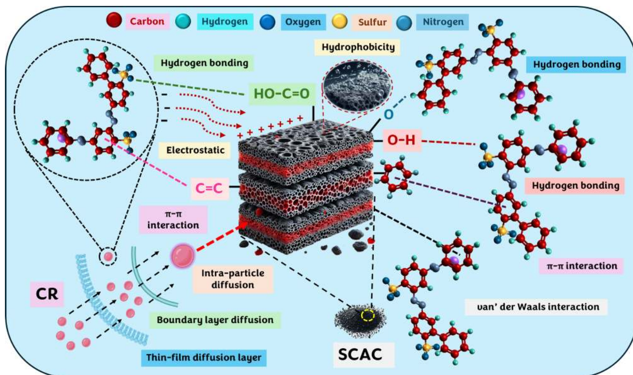
Fig. 9. Schematic representation showing the key interactions between SCAC and CR during the adsorption process.
