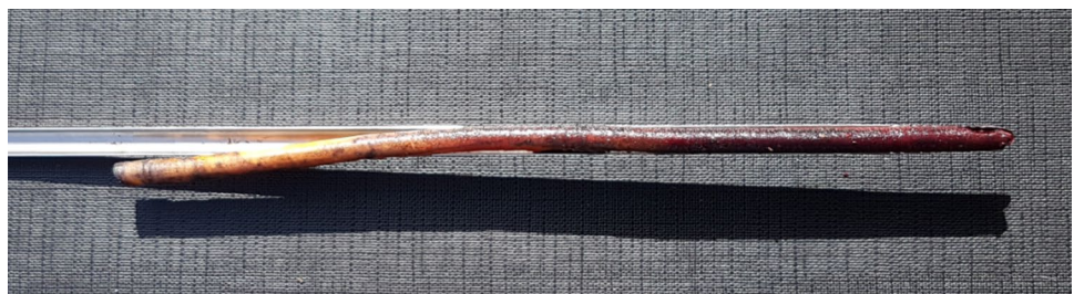
Fig. 4 Sapwood depth estimate using pH indicator dye in M. styphelioides (S1) tree grown in Bayswater Reserve
