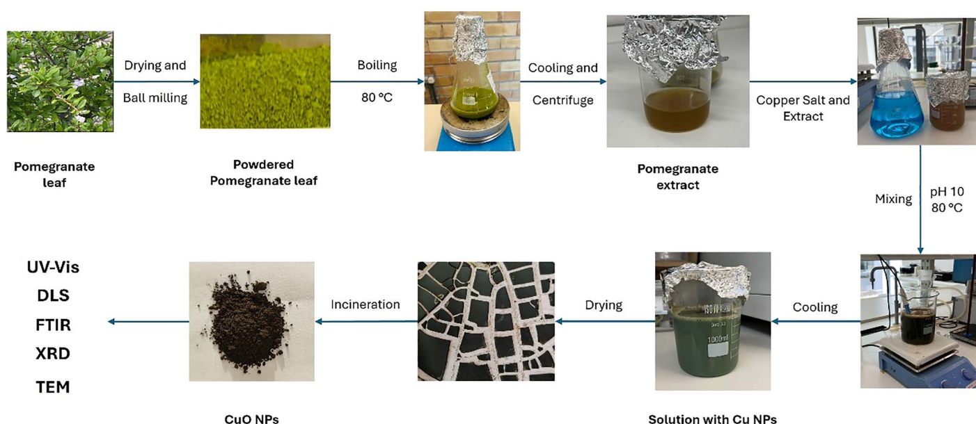
Fig 1. Punica granatum leaves and CuO nanoparticles synthesis procedure.
