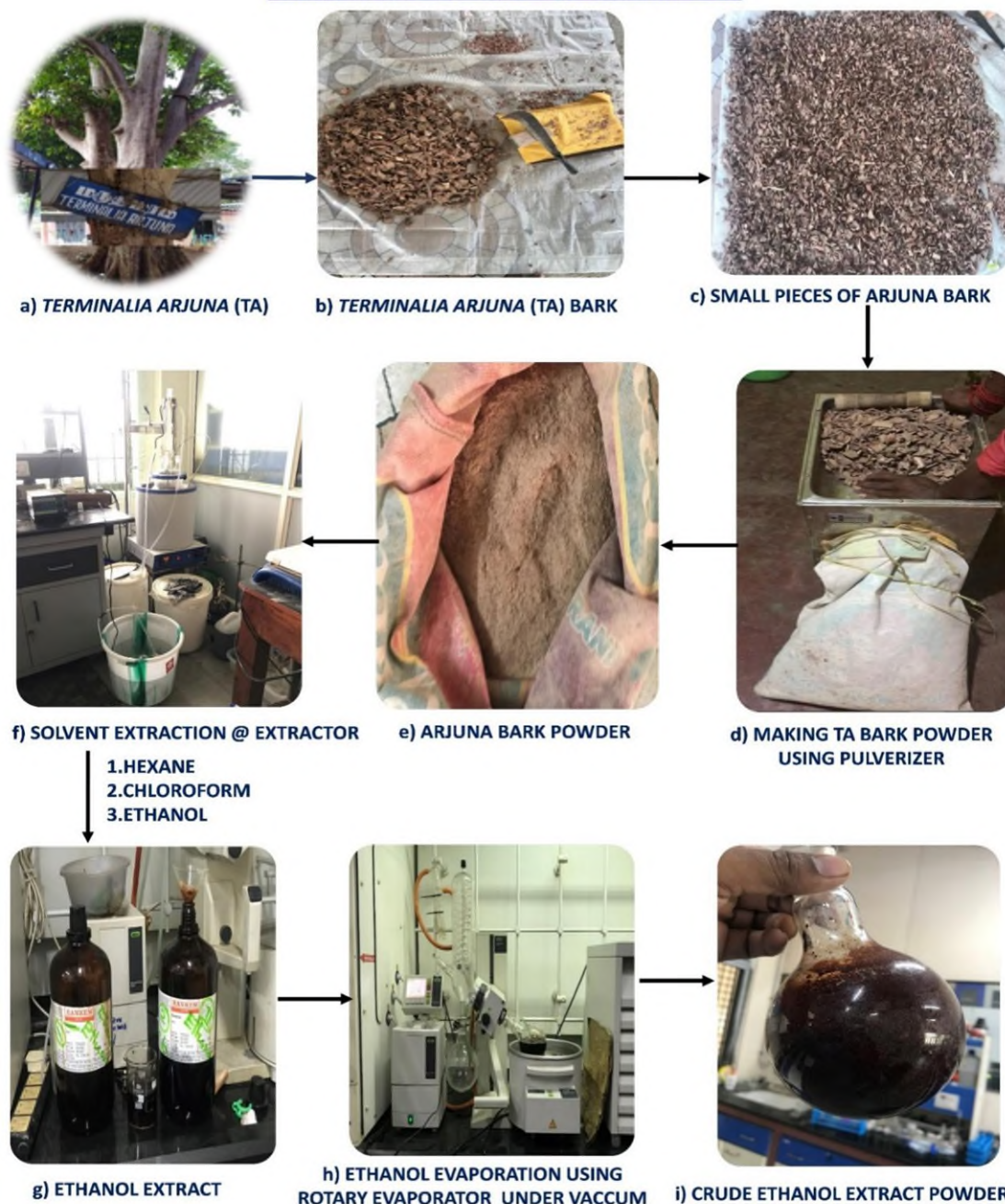
Figure 2. Extraction process of crude ethanolic extract from T. arjuna bark: (a) T. arjuna tree; (b) bark sample; (c) bark cut into small pieces; (d) pulverization of bark; (e) pulverized bark powder; (f) sequential solvent extraction using increasing solvent polarity (hexane, chloroform, and ethanol); (g) ethanolic extract; (h) solvent
