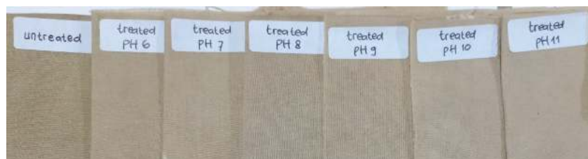
Figure 9. The effect of the in situ ZnO NPs immobilization process at various pH on the color quality of ND-colored Batik fabric.
