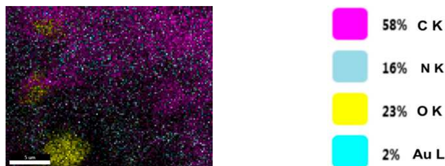
Figure 9. Engineered viscum–AuNPs carrier assembly: SEM—live map.
