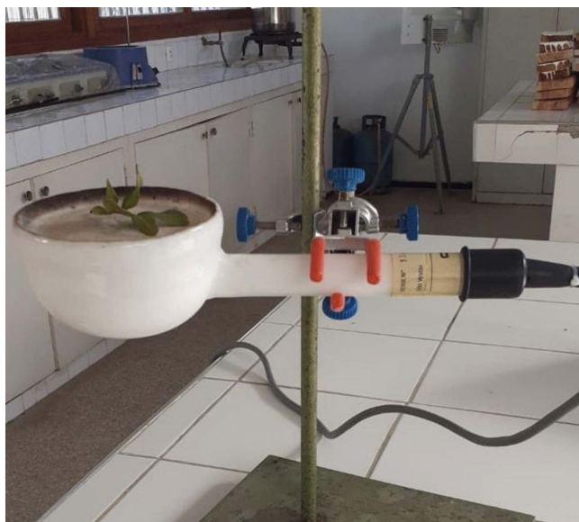
Fig 2. Photograph of the epiradiator used for twig flammability testing of fuel species in the laboratory.
