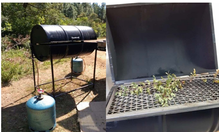
Fig 1. Photographs of the standardised grill used for field shoot flammability testing.
