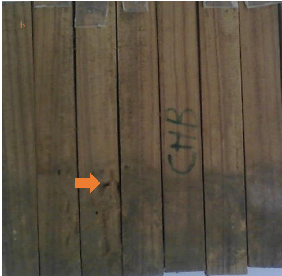
Plate 3.1: Coppiced P. erinaceus heartwood: Butt position after 12 months of field exposure (Arrow shows termite attack).
