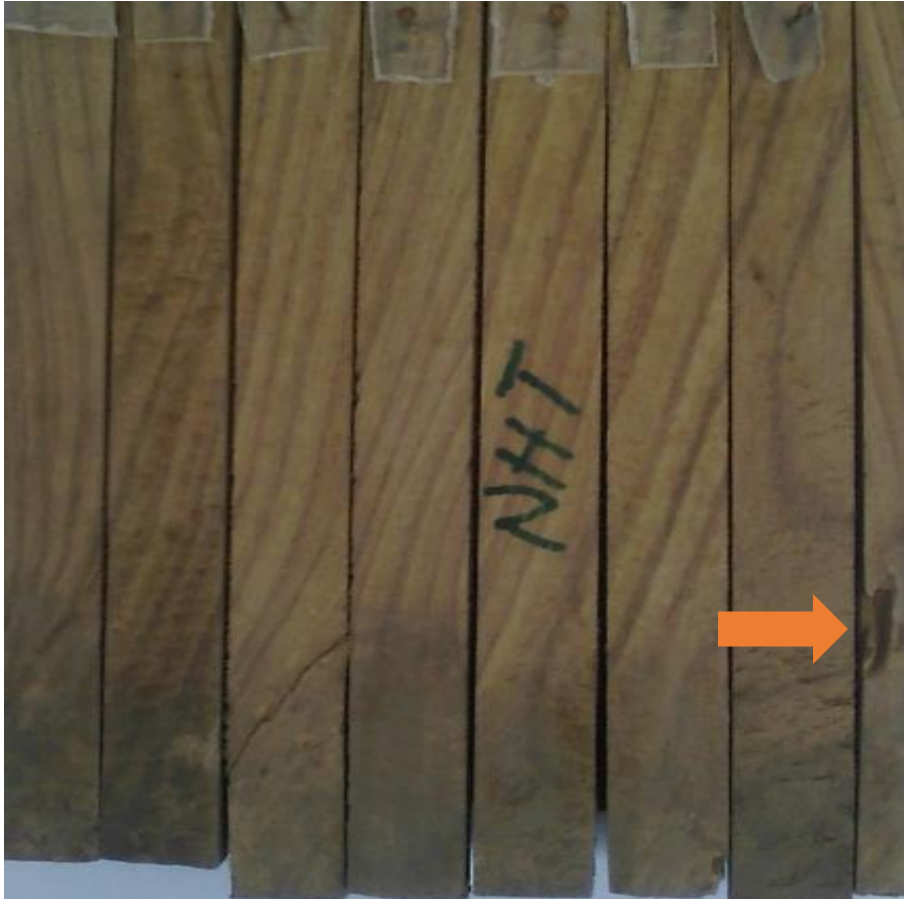
Plate 3.9: Non-coppiced P. erinaceus heartwood: Top position after 12 months of field exposure (Arrow shows minor termite attack).
