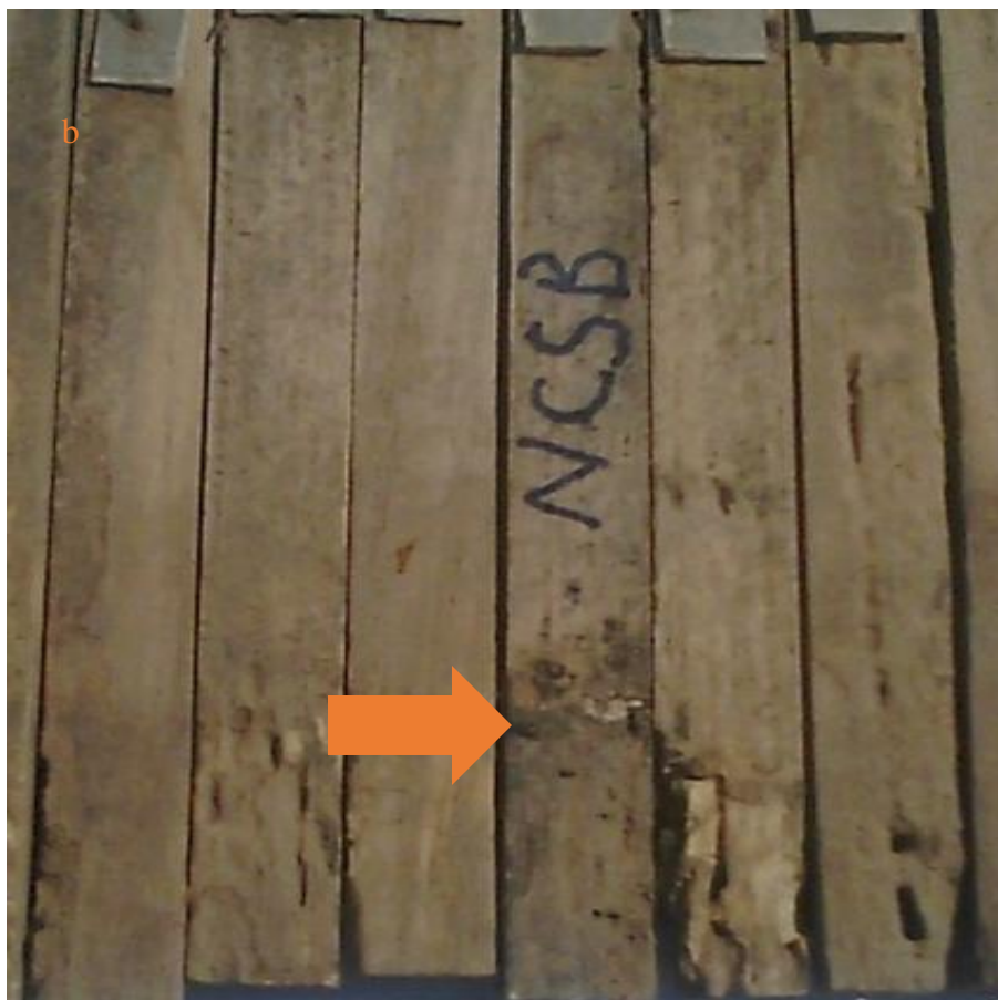
Plate 3.10: Non-coppiced P. erinaceus sapwood: Butt position after 12 months of field exposure (Arrow shows termite attack).
