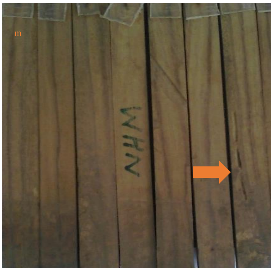
Plate 3.8: Non-coppiced P. erinaceus heartwood: Middle position 12 months after field exposure (Arrow shows minor termite attack).
