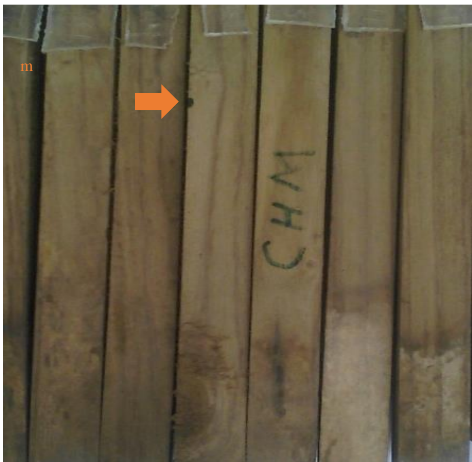
Plate 3.2: Coppiced P. erinaceus heartwood: Middle position after 12 months of field exposure (Arrow shows minor termite attack).
