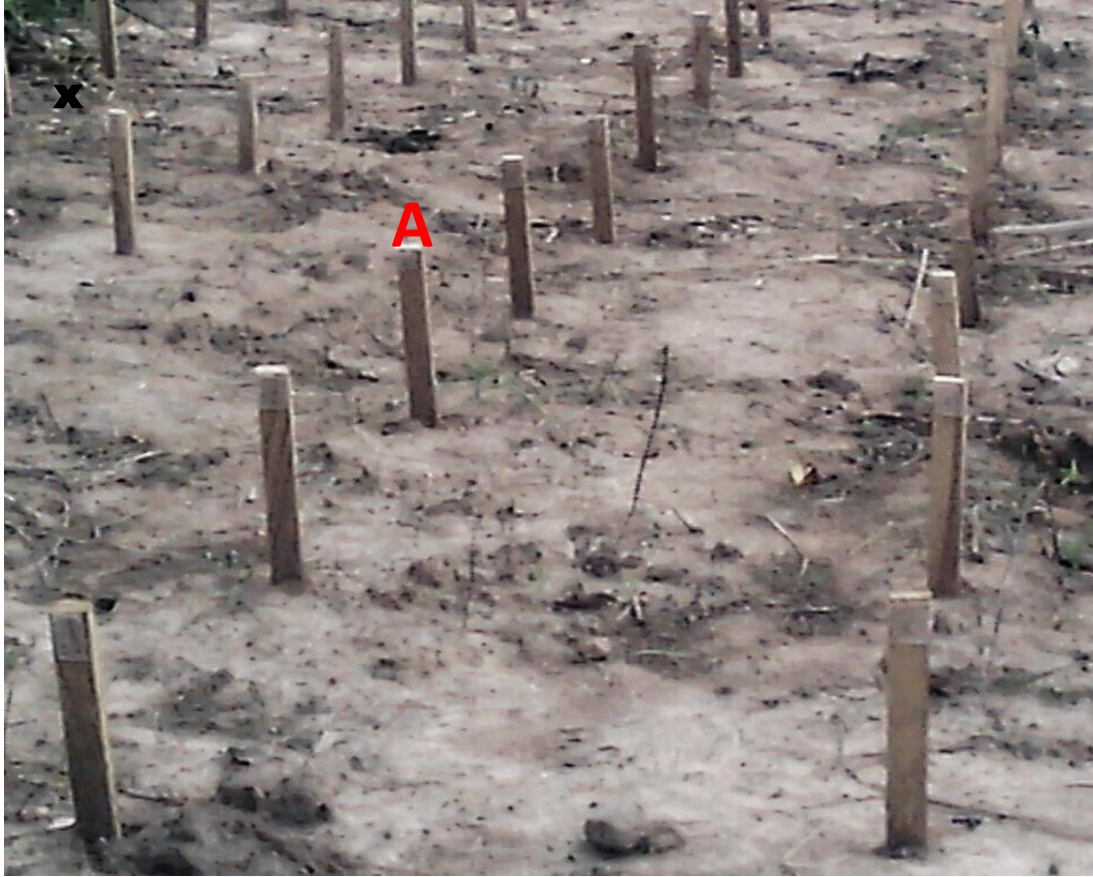
Plate 2.1: Stakes (A) implanted upright at the test site for durability assessment. Grid dimension: 50×60 m 2
