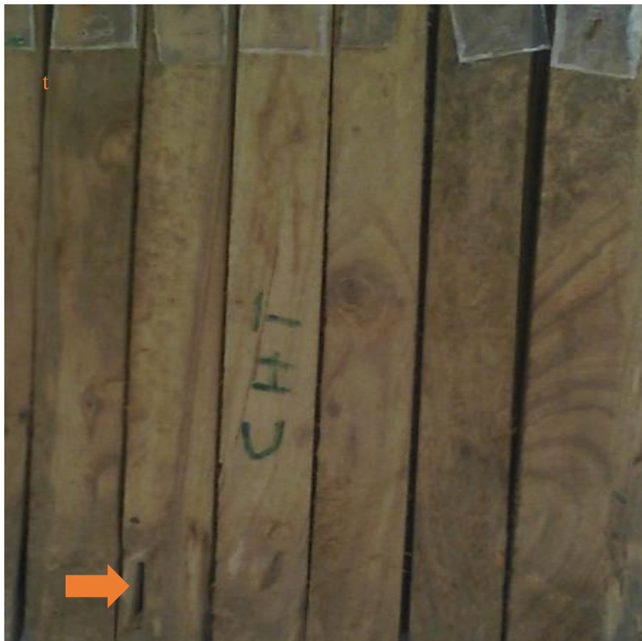
Plate 3.3: Coppiced P. erinaceus heartwood: Top position after 12 months of field exposure (Arrow shows termite attack).
