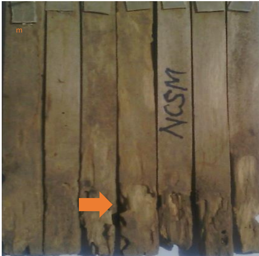
Plate 3.11: Non-coppiced P. erinaceus sapwood: Middle position after 12 months of field exposure (Arrow shows termite attack).
