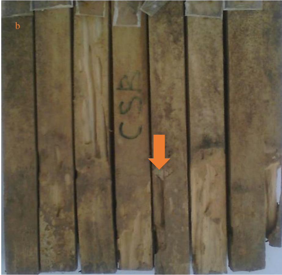
Plate 3.4: Coppiced P. erinaceus sapwood: Butt position after 12 months of field exposure (Arrow shows termite attack).
