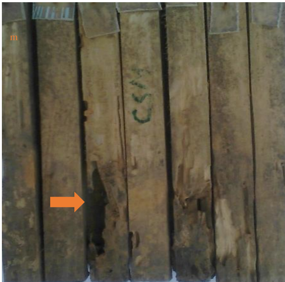
Plate 3.5: Coppiced P. erinaceus sapwood: Middle position after 12 months of field exposure (Arrow shows severe termite attack).
