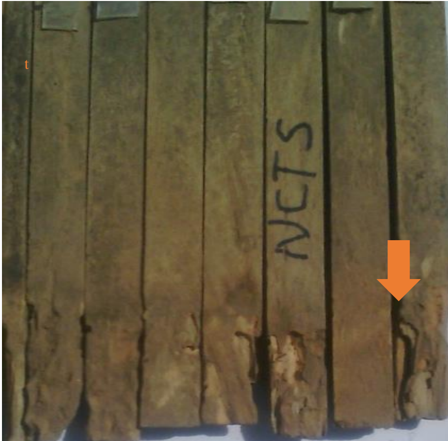
Plate 3.12: Non-coppiced P. erinaceus sapwood: Top position after 12 months of field exposure (Arrow shows termite attack).
