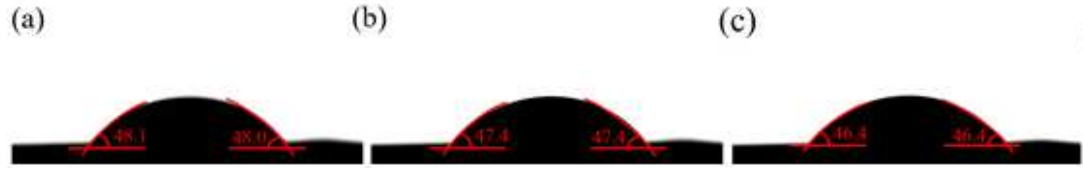
Figure 9 Static Contact Angle Measurement Results for Schima superba Leaves ((a) Test number 1; (b) Test number 2; (c) Test number 3)
