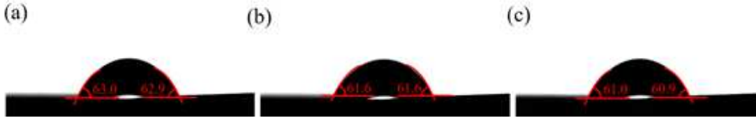
Figure 10 Static Contact Angle Measurement Results for Pinus massoniana Leaves ((a) Test number 4; (b) Test number 5; (c) Test number 6)
