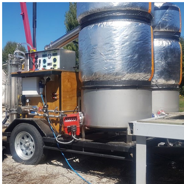
Figure 2. A mobile steam vacuum distil used for essential oil production in New Zealand.
